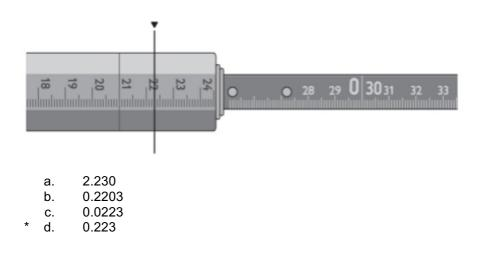
7.03 The tank was dipped using a sounding tape and shows the figures as below, what is the correct reading in metres if the oil cut is at the black line?
